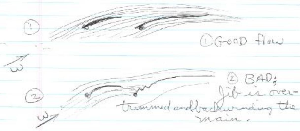
When close hauled or reaching, smooth flow (1) above) can be maintained until you head too far downwind. When running before the wind airflow becomes detached and the jib will be blanketed by the main.
