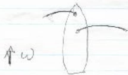
A caution when running downwind: Avoid "sailing by the lee" (carrying boom on windward side of boat). This could lead to a "goose-wing jibe" (an unintentional jibe when the wind catches the main on the back side and whips it across the boat) ☠
