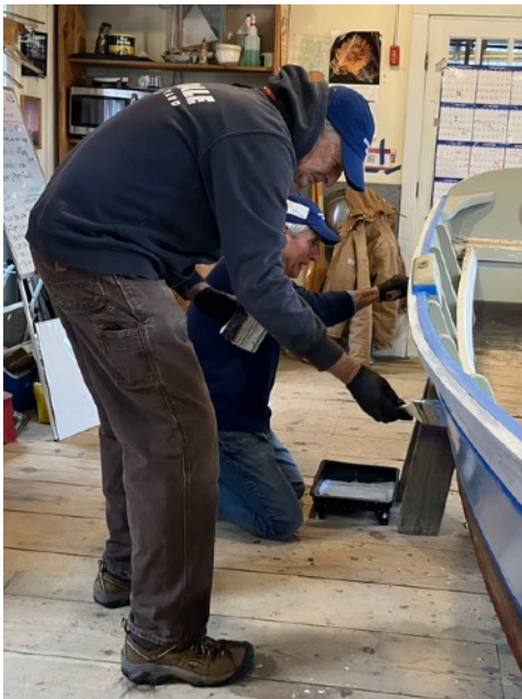
Al Grant rolling and Mac Cooper tipping topside paint on Culler punt “Skye”; Mac and John Malmros painting the inside of “Chuck” the popular Noank Skiff.
